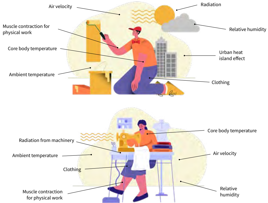
Fig. 1.2a: Illustration of the interaction of different occupational factors that can increase heat stress. Work demands dictate the internal metabolic rate, which is the major source of heat gain. Environmental factors and clothing determine the remaining avenues of heat exchange. The asterisk indicates that conduction and convection can lead to heat gain or loss; under most conditions, these are relatively minor avenues of heat exchange
